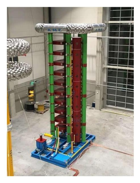
The impulse voltage generators are designed for testing high voltage equipment of power systems with lightning (LI: 1.2/50 μs), with chopping (LIC: 1.2/2÷6 μs) and switching (SI 250/2500 μs) impulses according to the IEC standard 60060-1 (IEEE, GOST, etc).
