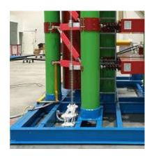
All our impulse generators are specifically designed to withstand disasters such as earthquakes.
